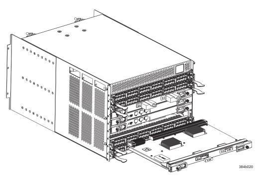
Figure 36. Removing and replacing the core switch blade
